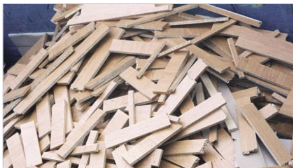
Off-cuts of MFC have limited uses other than for combustion with heat recovery
